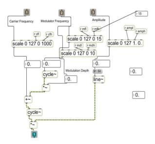
Figure 9: Frquency Modulation
